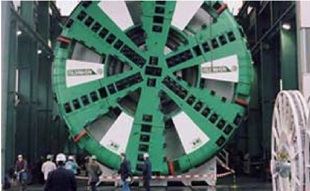
Dublin Port Access Tunnel, 11.7 m hard-rock TBM
